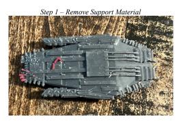
Using clippers and a file, remove the remaining 3D printed support material from the miniature. The above image shows some examples of support material highlighted in red. Your miniature will be a bit different. After removing this material, the little bumps where support material was attached to the miniature will need to be filed down.
